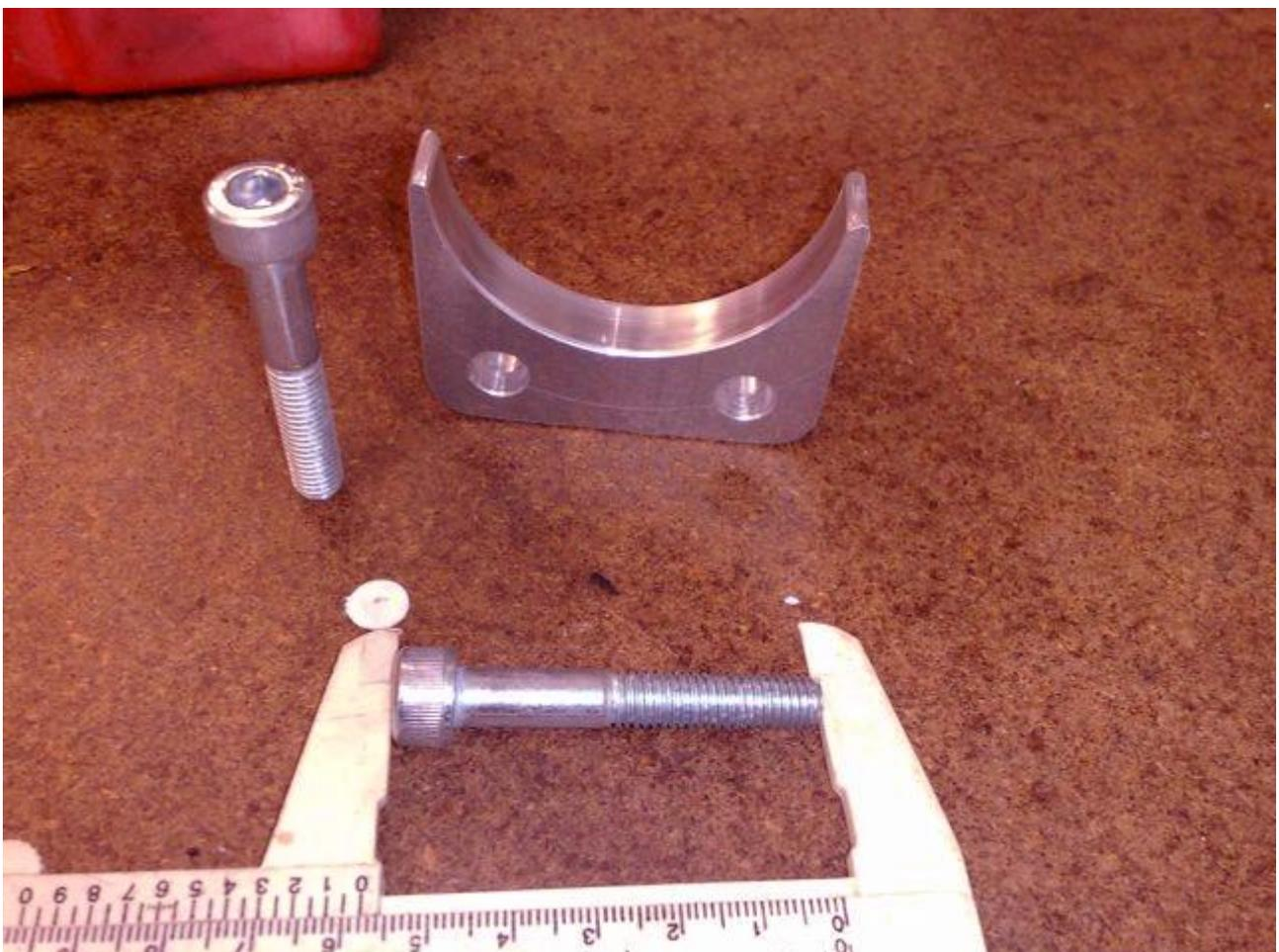
They sit in nice and tight against the machined face on the sliders and wrap around so they should be able to withstand the shear stresses they will have to transfer:
